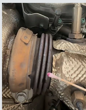
Positive chromium(VI) rapid tests in the engine compartment of passenger cars.
