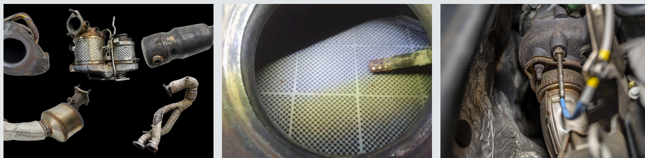
Typical used parts from the exhaust line; yellowish deposits on the particulate filter; sensor with deposits on the insulated exhaust pipe.
