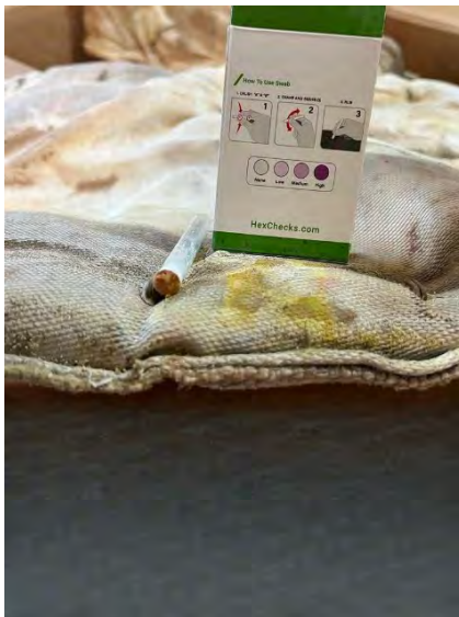
Fig. 60-64: Chromate deposits on insulating mattresses
