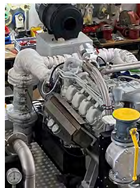
Fig. 70/Fig.71 Exhaust gas pipe CHP insulated calcium-free
