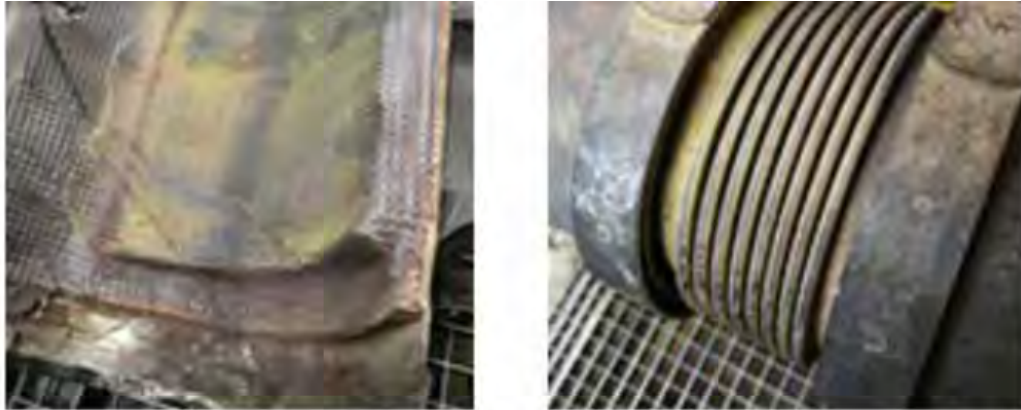
Illustration 1 Exhaust system examples of yellow residual deposits
