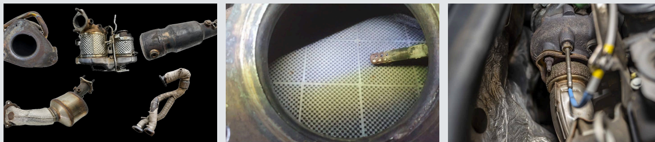
Typical used parts from the exhaust line; yellowish deposits on the particulate filter; sensor with deposits on the insulated exhaust pipe.
